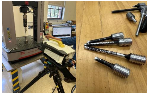
Figure 1. Left: The experimental setup described in this abstract including the MTS tensile test unit, and the Telops FAST M3k. Right: Fractured aluminum (center) and steel (upper right) samples imaged after testing.
