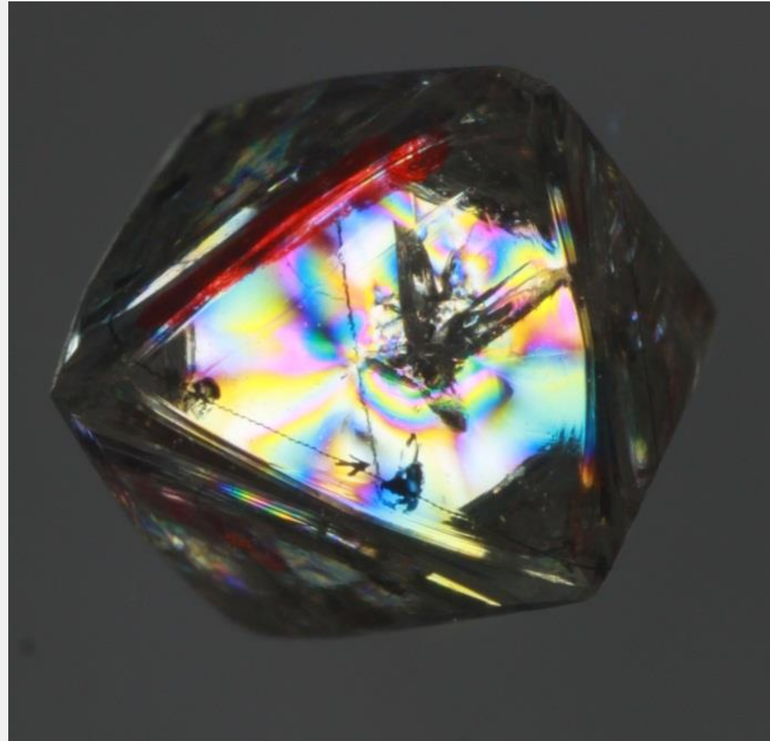
Residual stresses in an uncut diamond
