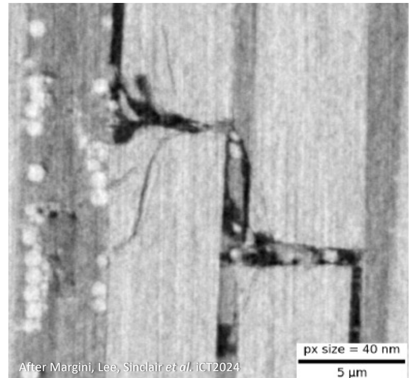
After Margini, Lee, Sinclair et al. iCT2024 CFRP fibre fracture & DVC, 40nm resolution
